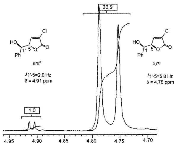
**Figure 2.** >20:1 *syn/anti* mixture of 3-chloro-5-(1'-hydroxy)-furan-2(5H)-ones: resonance of proton on the C1' after D<sub>2</sub>O addition.
